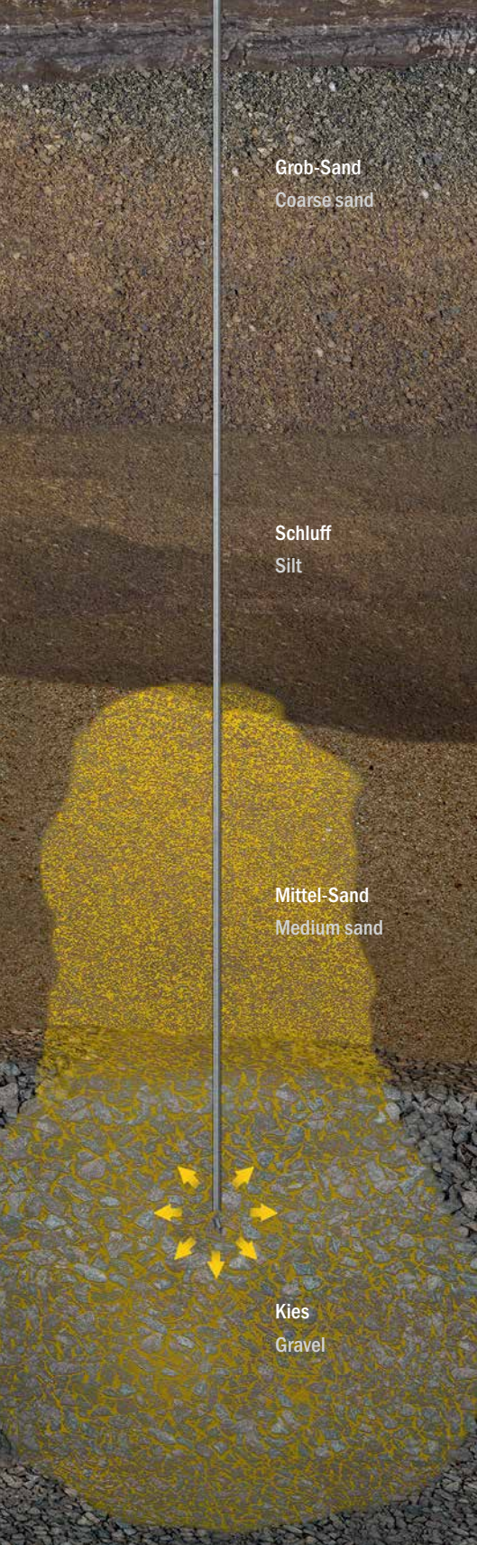
Detail: Verlorene Spitze Detail: Separated tip
