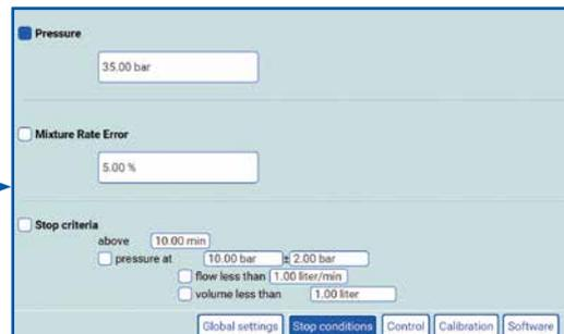
All marked DESOI w.i.l.m.a.'s can be upgraded to the PRO version. The PRO version contains an additional cancellation criteria and electronic pressure control.
